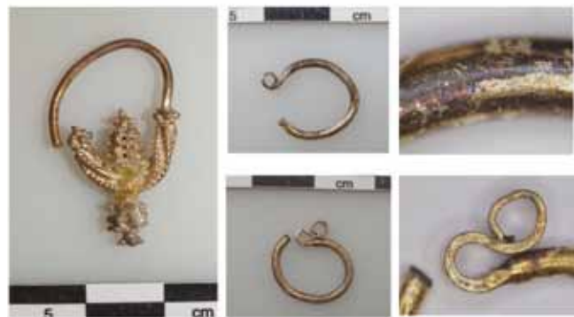
Fig. 1 Example of earring and temples rings prior treatment, covered by a thin tarnish layer of variable thickness and color
