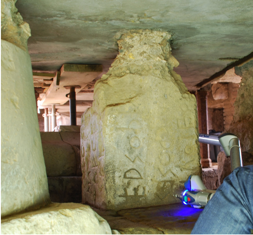
Fig. 2. The laser scanning of the Forum Cippus (July 3rd, 2015) with the CAM2 ARM device by FARO. Photo by M. Muscariello.
