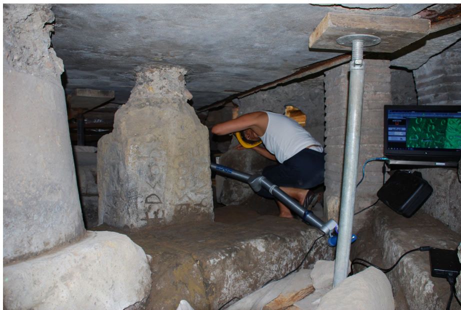
Fig. 4. A moment of the laser scanning. The articulated arm of the CAM2 ARM device is visible, as well as the computer that was showing the first results of the scanning. Photo by M. Muscariello.
