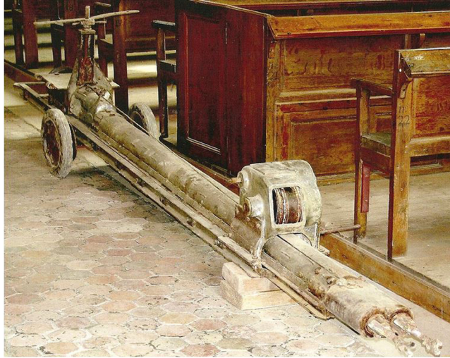
Figure 6: Machine à four with rotating drill bits – Roches & Carrières Archives.
