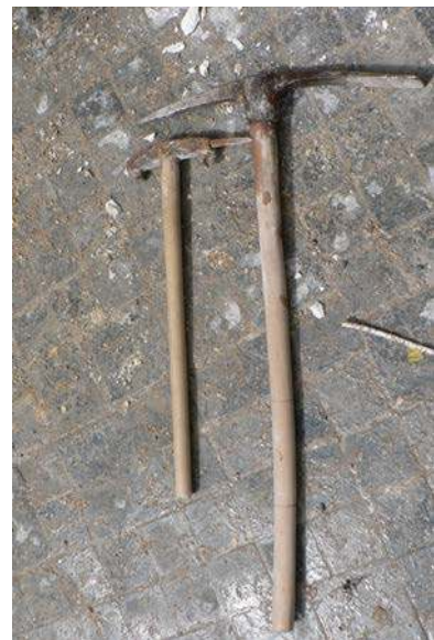
Fig. 10 A long-handled pick and a short-handled pick held by stonemason K. Manap (A. Lamesa).
