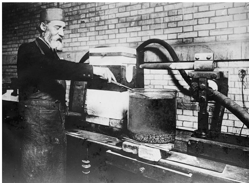
Fig. 3.1.2. Unknown author, Henri Moissan using a Moissan-Chaplet electric arc furnace. Credit: Wikimedia Commons.
