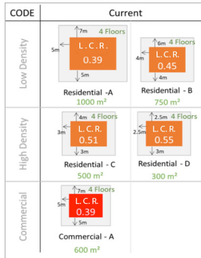
Fig. 5. 2. Building Regulation Codes
