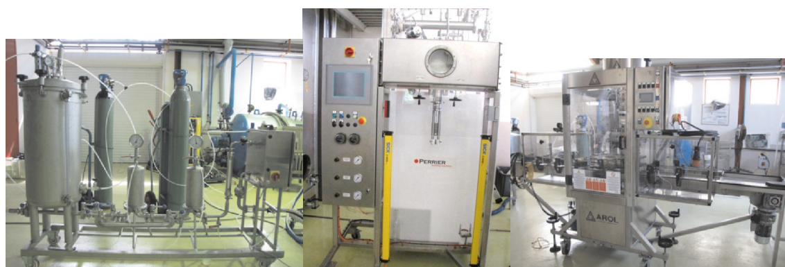
Figure 1. The three elements of INRA Pech-Rouge bottling line for experimental wines: filtration skid + filling and corking machines.
