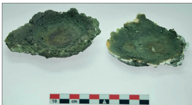
Fig. 7. Experimental litharge cake. Obr. 7. Lithargit z experimentů.
