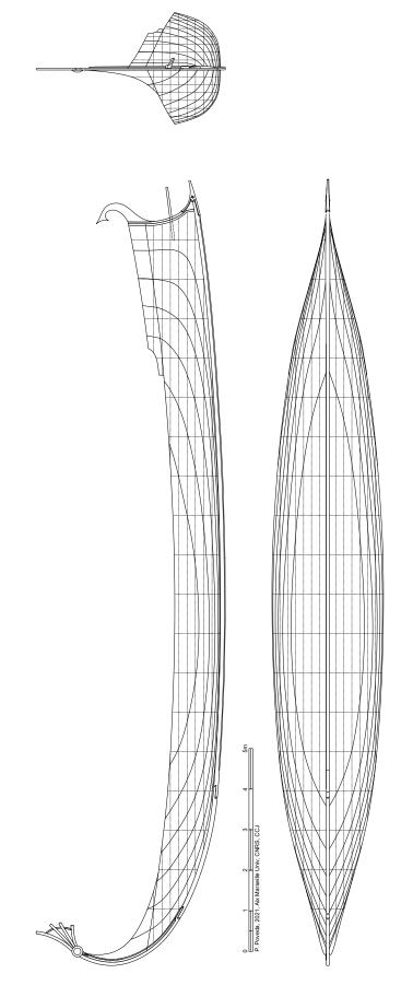
Fig. 8 Lines plan of the reconstruction (drawing: P. Poveda, CNRS, CCJ)
