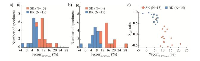
Figure 5: Histograms of cooling rate correction factor %corr for 0.8°C/min (a) and 0.4°C/min (b), cooling rates from 650°C for SK bricks and from 555°C for BK bricks; (c) S<sub>300</sub> ratio versus cooling rate correction factors (0.8°C/min slow cooling).
