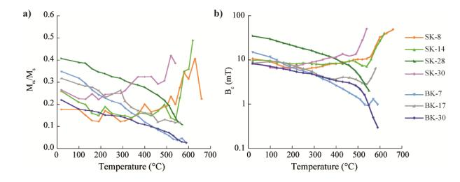
Figure 3: Variation with temperature of (a) the remanence ratio (i.e. the ratio of the saturation remanent magnetization  $M_{rs}$  upon the saturation magnetization  $M_s$ ) and (b) the coercive force  $B_c$ .
