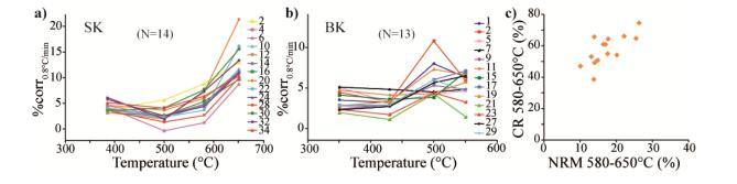
Figure 8: Variation of the cooling rate correction factors (0.8°C/min slow cooling) with temperature in SK (a) and BK (b) bricks. (c) For SK bricks, fraction of NRM demagnetized in this temperature interval versus percentage of the correction factor in the temperature interval 580-650°C.
