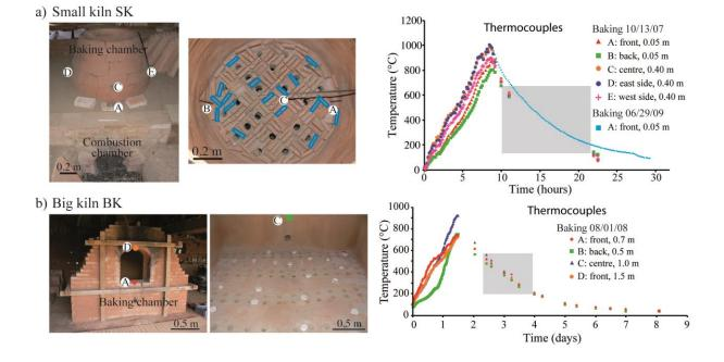
Figure 1: Photographs and heating-cooling temperature curves of the two experimental kilns a) SK small kiln and b) BK big kiln. The 17 sampled SK bricks are surrounded in light blue. The BK bricks were oriented *in situ* using the plaster cap method. The distance in meters associated to each thermocouple is the height above the plate. On the curves, the grey area indicates the time needed for the temperature to decrease in the range of unblocking temperatures of bricks.
