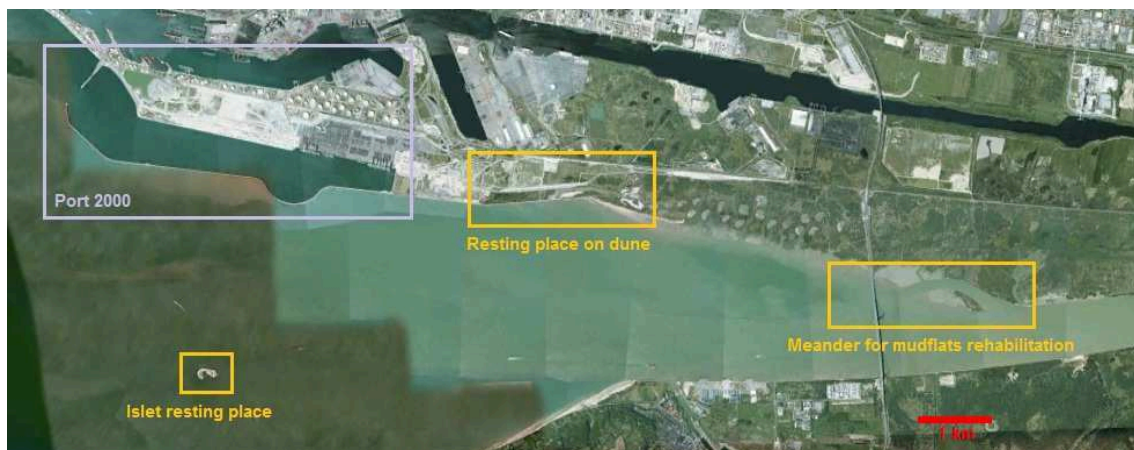
Figure 70 - Aerial view of Port 2000 and the environmental measures accompanying the project (Image: Google Earth - Cnes/Spot Image 2013)
