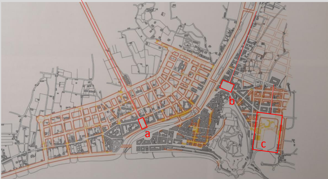
Figure 87 The city of Nice (grey) and the new plan of the Consiglio d'Ornato (orange) using squares with a key role for the street grid organisation: A) Place Massena; B) Place Garibaldi; C) Port Lympia. (Source Graff 2013)
