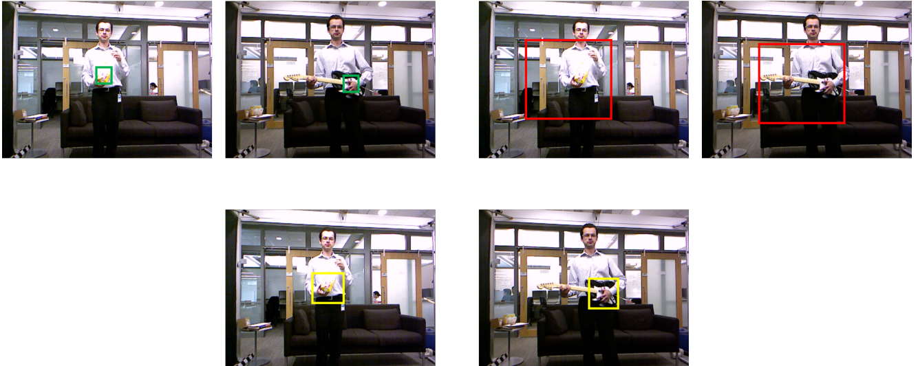
FIGURE 3.20: The illustration of object cube size. In the first row, the green rectangular and red rectangular represent small and large cube respectively. The yellow rectangular in the second row represent the appropriate size of object cube.
