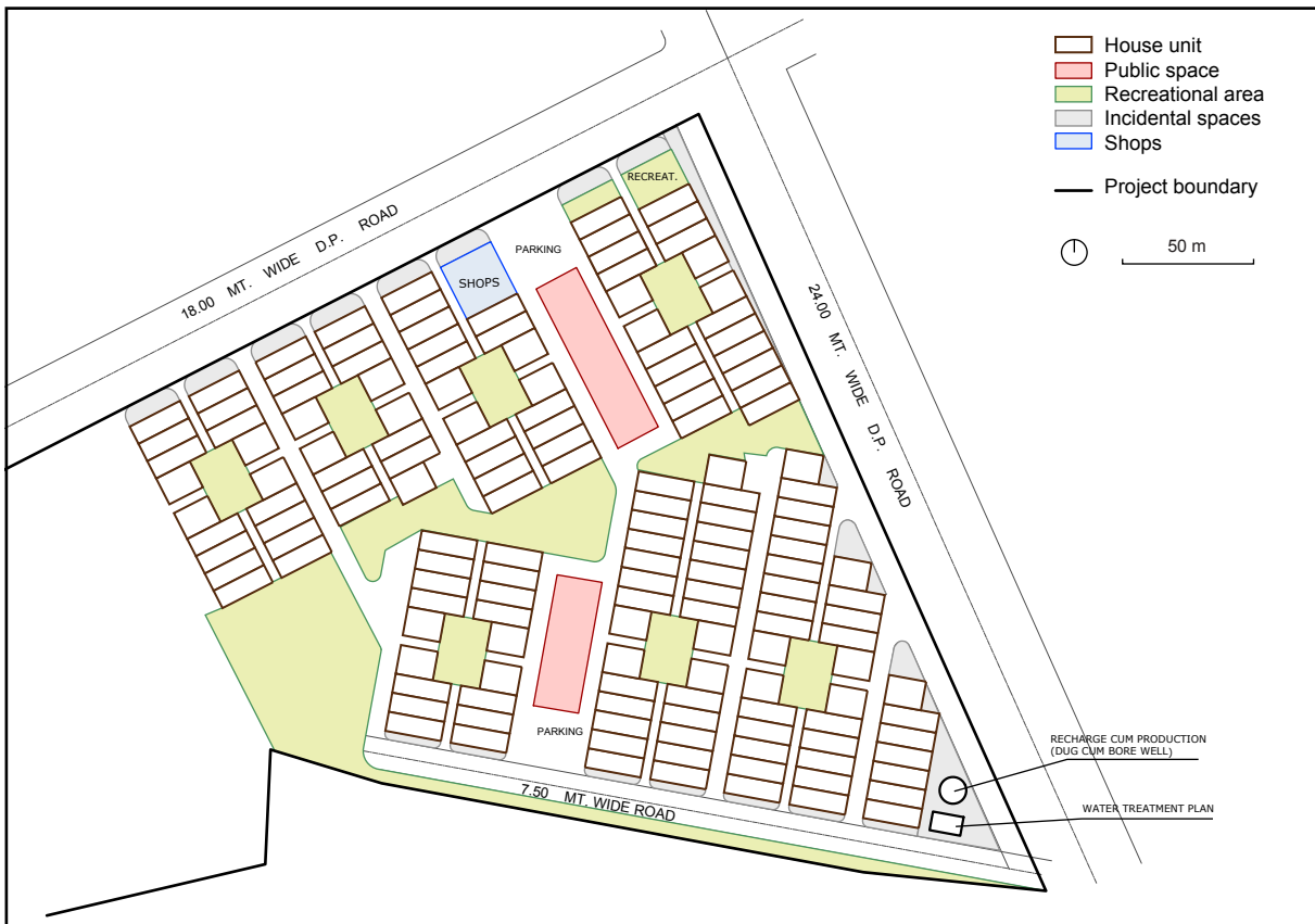
Site Layout for GIDC Relocation Site
