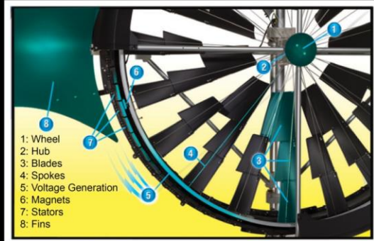
Blade Tip Power Production the magnets, and copper stators on the tip of the blade are producing a 'flywheel' effect.
