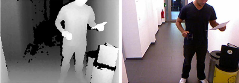
Fig. 9.16 — Carte de profondeur fournie par le capteur Kinect (source : [http://openframeworks.cc/ofBook/chapters/image\\_processing\\_computer\\_vision.html](http://openframeworks.cc/ofBook/chapters/image_processing_computer_vision.html)).
