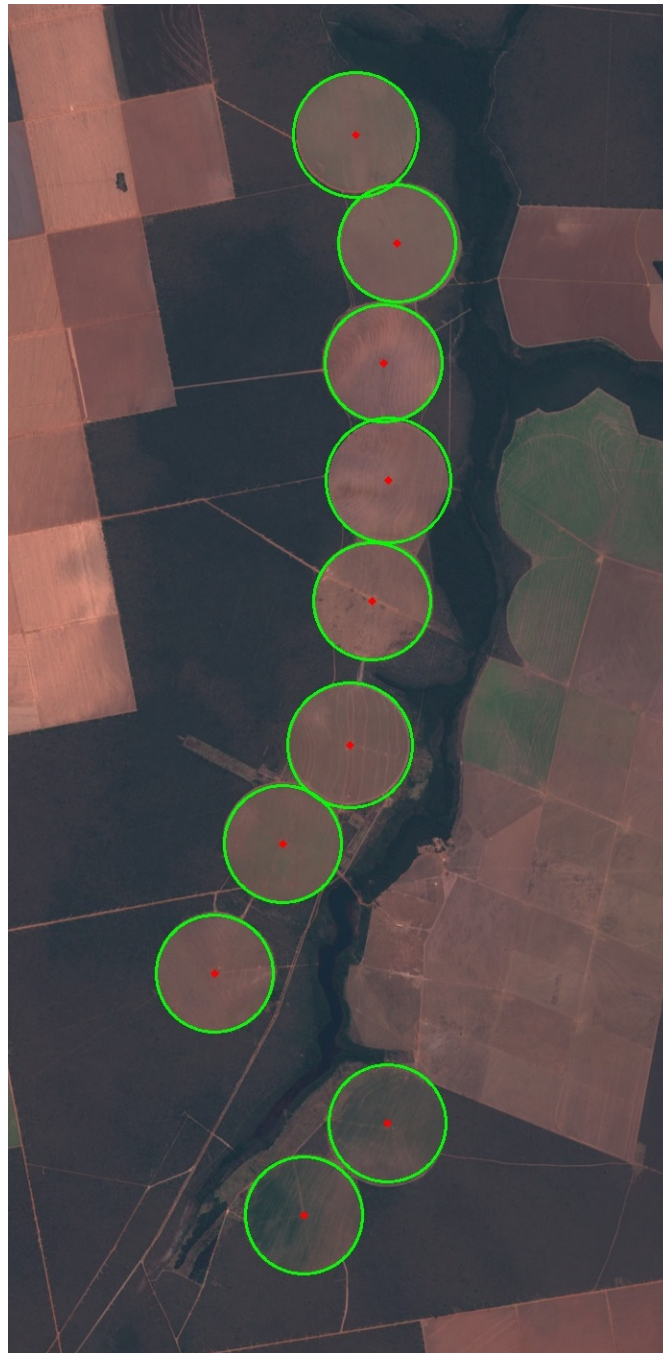
FIGURE 3.3: Automatic detection of center pivot irrigation systems on Sentinel 2 images [57].
