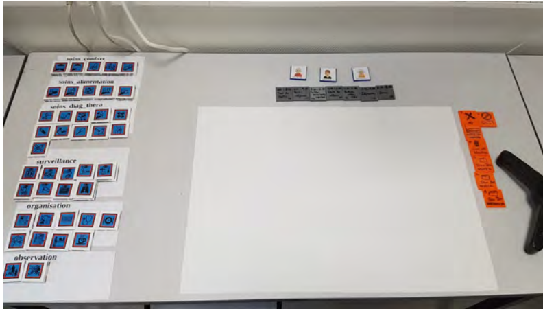
Figure 4.16: Table with the tokens' placement around the main interface that is projected on the blank paper at the centre. The paper is used to maximise light reflection as projector can be lacking in light intensity. Using it help keep the conditions similar across test sites.
