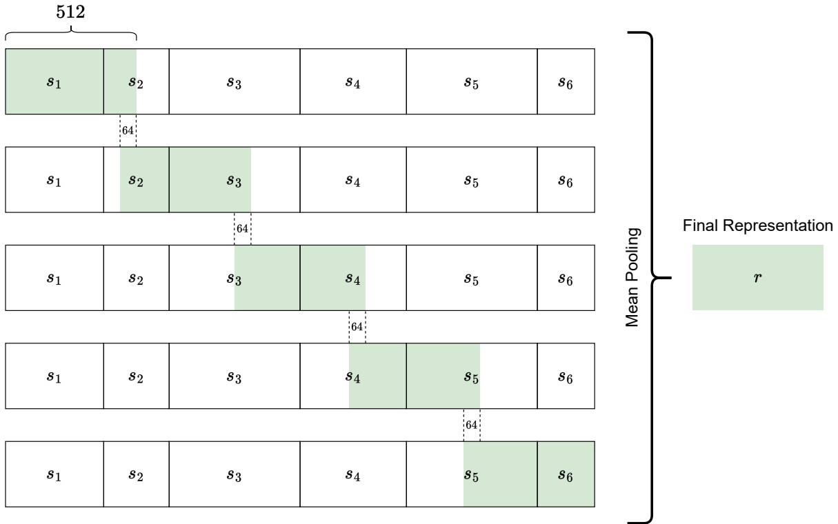
Figure 3.3: Illustration of the sliding window approach. A document x is composed of sentences s_i . We use a sliding window of size 512 with an overlap of 64, which means that we compute the representation of the first 512 tokens in the document, then the next 512 with an overlap of 64 on the first window, and so on until we reach the end of the document. All the representations obtained using this method are then aggregated using a mean pooling operation to obtain one final representation of size 512.
