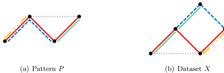
Figure 2.4: Illustration of the SIAM algorithm for finding the exact and partial matching of P in X , both represented by the dots. Each colored dotted line indicates a sub-pattern of P of at least two points that has been matched in X without redundancy (adapted from Meredith et al. [Meredith 2002a]).
