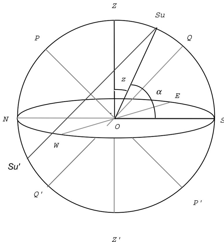
arc  $ZSu$ ) is called the Zenith distance of the Sun ( $z$ ). The angular distance between the Horizon and the Sun at  $Su$  is the altitude of the Sun ( $a$ ).
