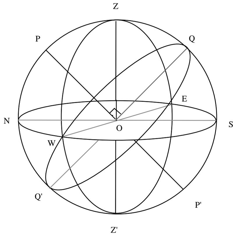
to two points on the surface of the sphere defines respectively the Zenith ( $Z$ , *nata*), which is the point above, and the Nadir ( $Z'$ ), which is the point below. This is illustrated in Figure 1.1.
