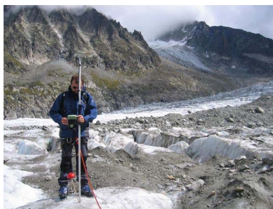
Figure 4. Rapid static GPS measurements (Mer de Glace)
