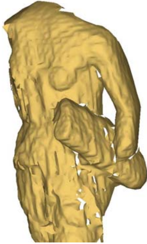
Figure 4. Best surface triangulation applied on the point cloud of figure 3
