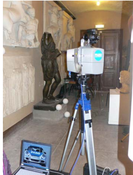
Figure 2. The TLS and the statue to digitize.
