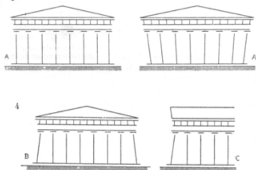
Figure 3: Choisy’s drawings do not correspond to the real geometry of Greek compositions, but provide a real information to the reader: top, right, the illusion of divergence that the human eye naturally perceives, bottom, the corrective disposal adopted by ancient Greeks.
