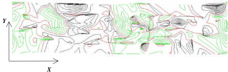
Figure 6. Intrados cylinder least square optimization with 20x anamorphosis of residuals. : iso-deformation curve (each 5 cm) from the computed Cylinder. In green out of the cylinder, in black inside the cylinder.
