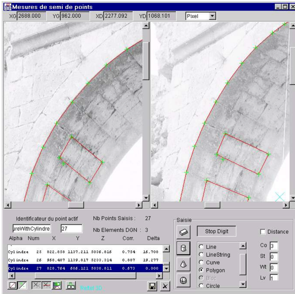
Figure 3. Aleyrac project : Semi-automated Primitive Measurement Method applied to a cylindrical shape.
