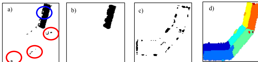
Figure 2. a) DSMb of the detected plane (yellow plane in Fig.2d); b) DSMb of the improved detected plane; b) DSMb of the remaining points after detecting the roof planes; d) Final result of roof planes detection.
