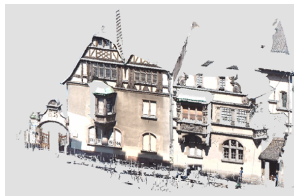
Fig. 14. Point cloud (raw data) displayed with true color pixels
