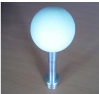
Fig. 6a: Target spheres with forced centring device
