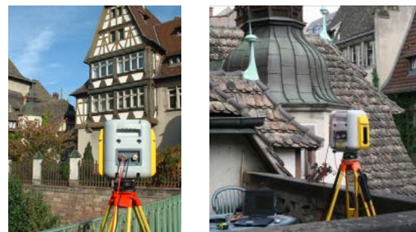
Fig. 10. Trimble GX scanner during the survey
