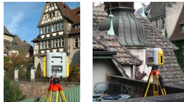
Fig. 10. Trimble GX scanner during the survey
