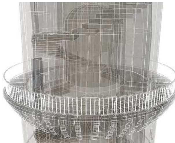
Figure 4: A partial view of a 3D model of the signal light tower, showing the balcony on level 3 and the spiral staircase (UMR MAP, 2006).
