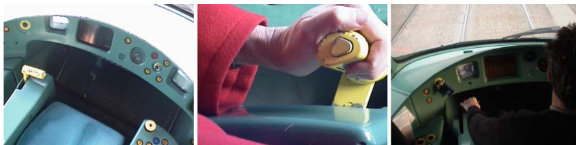
Figs. 9–11 Eurotram control cab—throttle, alarm and dead-man—action on the throttle
