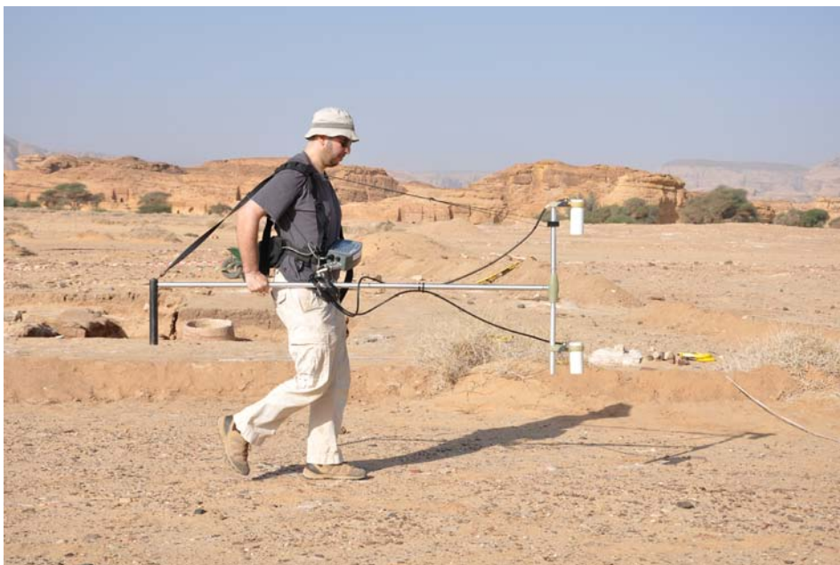
Fig. 2. The G-858 Cesium magnetometer (Geometrics) used in Madâ'in Sâlih
