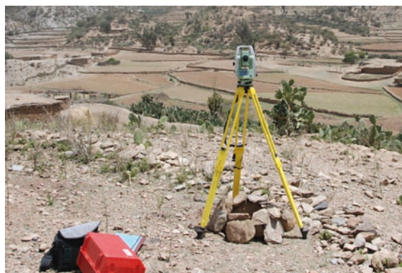
Figure 3: Total station Leica Flexline TSo6 (IG 2011).
