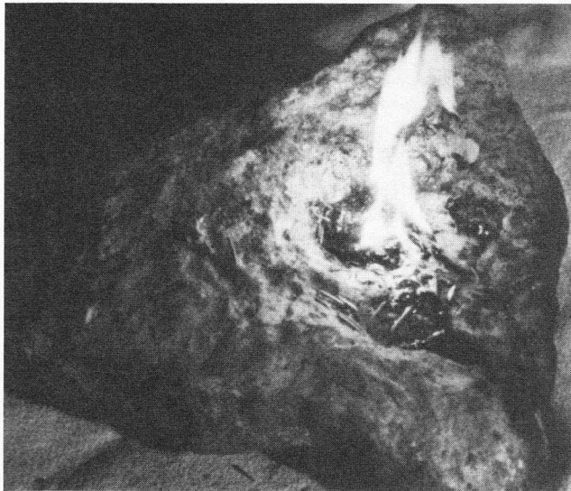
Figure 5. Experimental limestone lamp with the cavity opening on the side, using equid fat and juniper. 252 x 197 mm (photo S. A. de Beaune).
