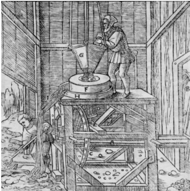
Figure 19. Representation of an ore mill according to Agricola.
