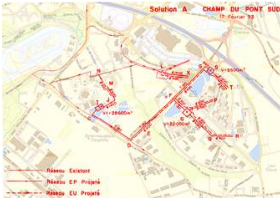
Figure 16. Draft of the stormwater management system for the Technology Park as established by Greater Lyon (Grand Lyon, 1993) 1 .
