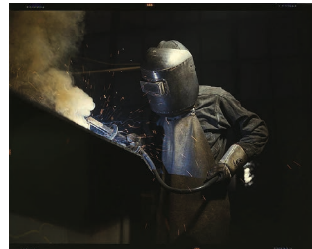
Welder making boilers for a ship, Combustion Engineering Company. Chattanooga, Tennessee, June 1942. Reproduction from color slide. Photo by Alfred T. Palmer. Prints and Photographs Division, Library of Congress.
