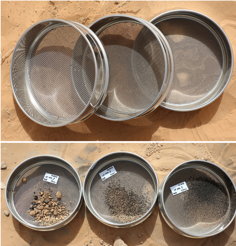
Figure 123: The column of the geological sieves (up) and the different refuses of sediment after sieving stage (bottom) (Ch. Bouchaud - Saudi French archaeological mission in al-Kharj).
