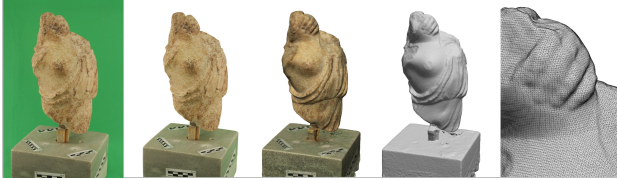
Figure 6: Different steps of the image processing: Raw photograph; clipped image; colored 3d mesh; raw mesh; mesh detail.
