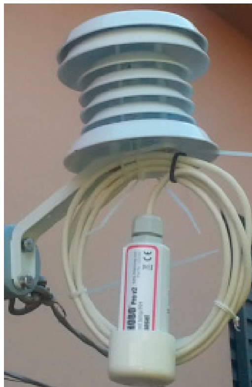
Figure 6. Meteorological shelter (type RS3-HOBO) with temperature and humidity recorder featuring external probe—U23-002 data logger—HOBO.
