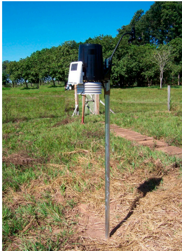
Figure 7. Davis Instruments Vantage Pro 2 weather station.
