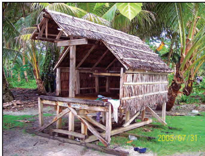
Figure 2: Manned Indonesian fish aggregating device (FAD) washed ashore on Mwooch Island, Chuuk State, after a storm
