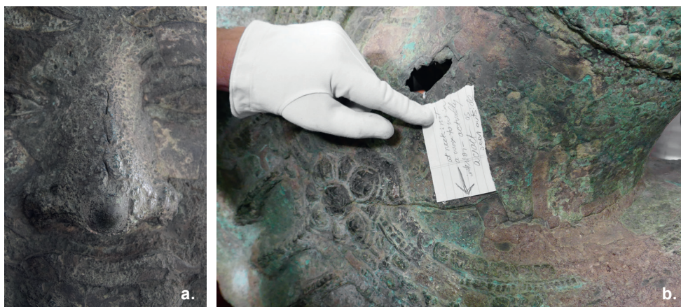
Fig. 25 — Examples of casting flaws ( ga 5387): (a) detail of the nose; (b) back of the neck.
