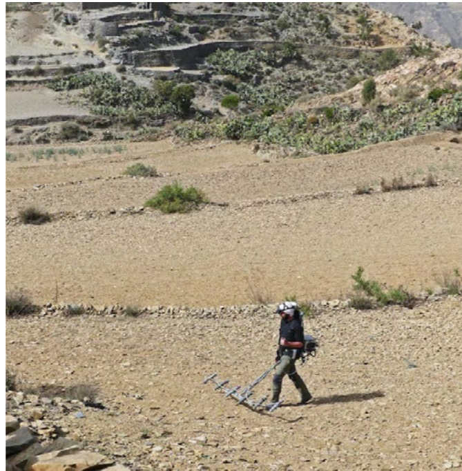
Figure 2: Measuring device developed by IPGS with six magnetometers (N. Blond – MAFTOr).
