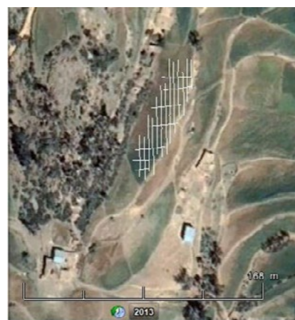
Figure 8: Profiles and tie-lines on terrace 2 (R. Al Khatib Alkontar, H. Reiller – MAFTOr/IPGS-EOST).
