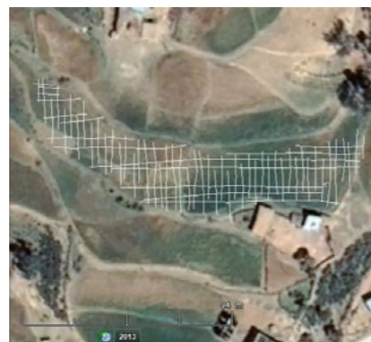
Figure 7: Profiles and tie-lines on terrace 1 (R. Al Khatib Alkontar, H. Reiller – MAFTOr/IPGS-EOST).
