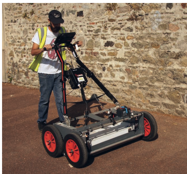
Figure 1. Geophysical devices used during the survey: a) Electrostatic “sliding carpet”, b) Electrostatic MP3, c) IDS Georadar (Stream X V8).
