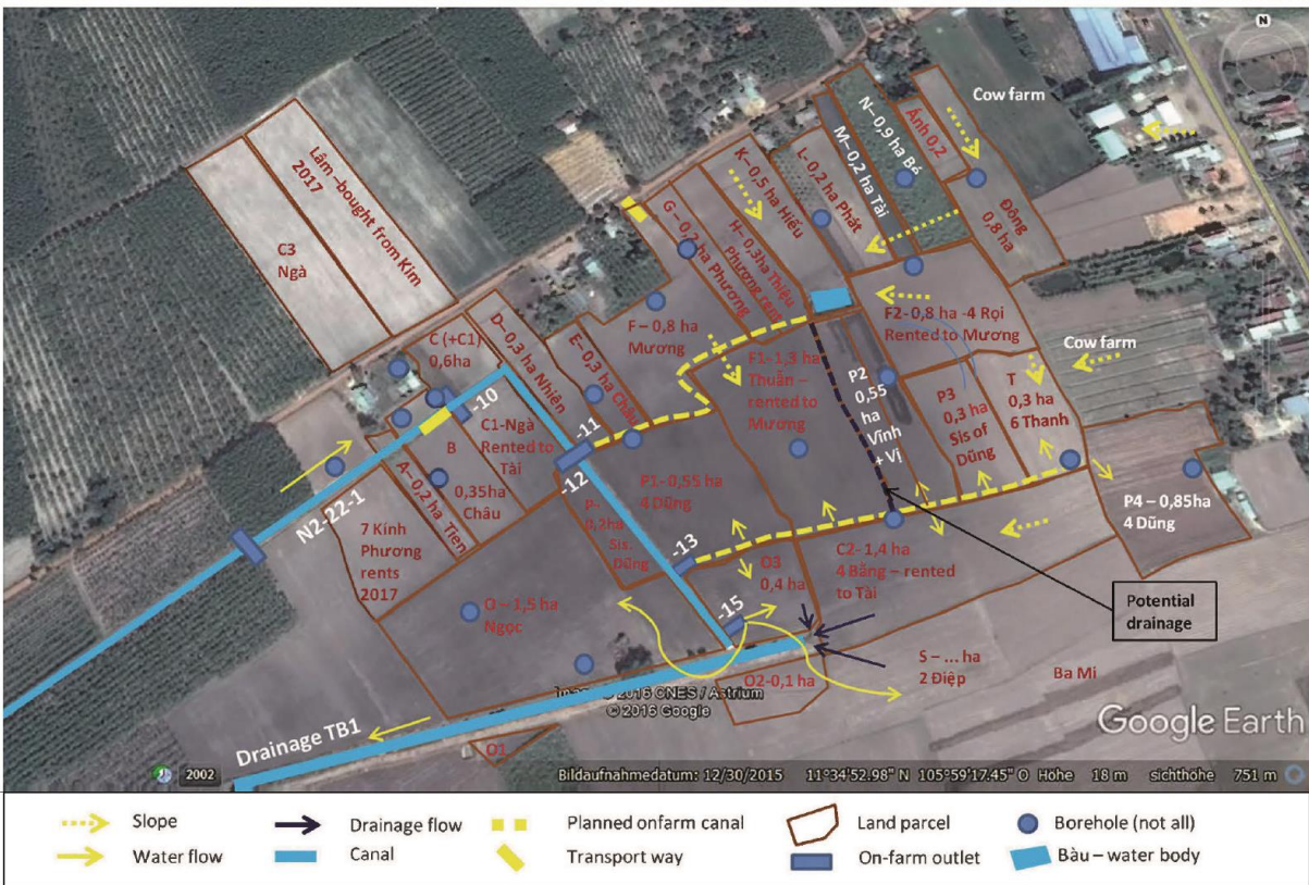
Top left: Collective work to build an on-farm canal on March 19, 2017; Top right: Canal N2-22-1 in February 2017; Bottom: Layout of canals and land parcels in December 2017. Source: EFEO, 2019.
