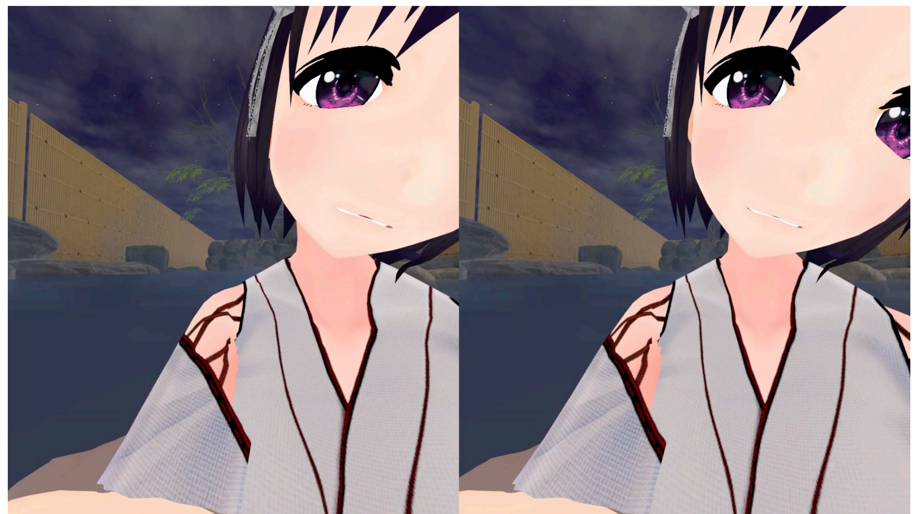
Image 1. Image 1. Co-founder Karin in a virtual environment. For the VR goggles solution, two images, one for each eye, are streamed on the phone positioned inside the goggles at 5Mbps using VP8/9
