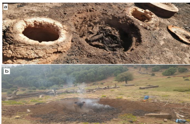
Figure 14: Photo of site of tar production (a) in Talgout (Excavated indirect-fired); (b) In Itzer (Charcoal kiln Direct fired) (Taken by Ninich Oumaima)
