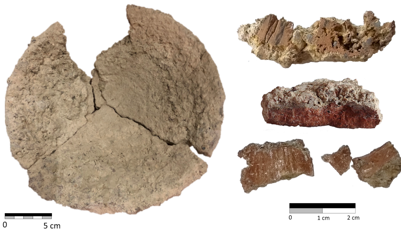
Fig. 2. Plan view, left: macroscopic appearance of litharge cakes from Las Tres Hermanas; cross-section, right: top – sawn surface of a porous litharge (Las Tres Hermanas), middle – highly altered surface of a non-porous litharge (Las Tres Hermanas), bottom – a fragment of litharge (altered surface) from the Campello site (La Illeta dels Banyets).
