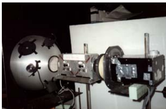
Fig. 2.3.: Calibrating the aircraft version of POLDER with the sphere. http://www-loa.univ-lille1.fr/Instruments/fr/polarimetres/polder/carac.php
